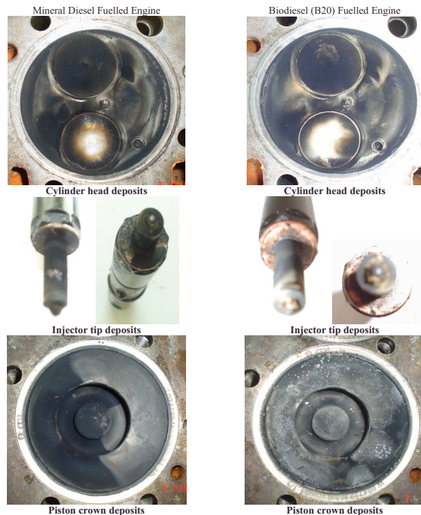
Fig. 2 Carbon deposits on vital engine parts
