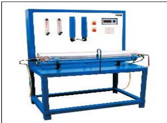
Fig. 6. Experimental setup of the double pipe heat exchanger
