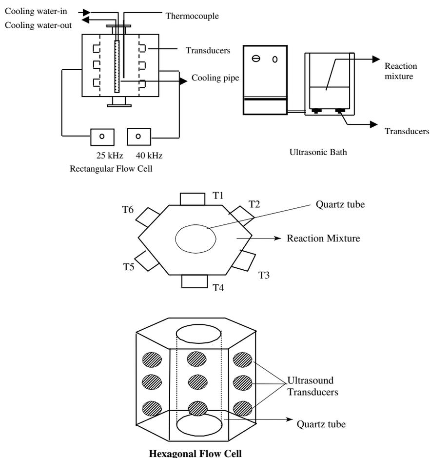
Figure 1. Multiple transducer based sonochemical reactor.
