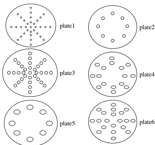
Figure 3. Multiple hole orifice plates having different combinations of number and diameter of holes.
