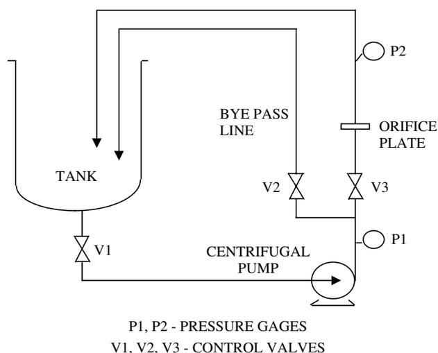
Figure 2. Orifice plate hydrodynamic cavitation setup.
