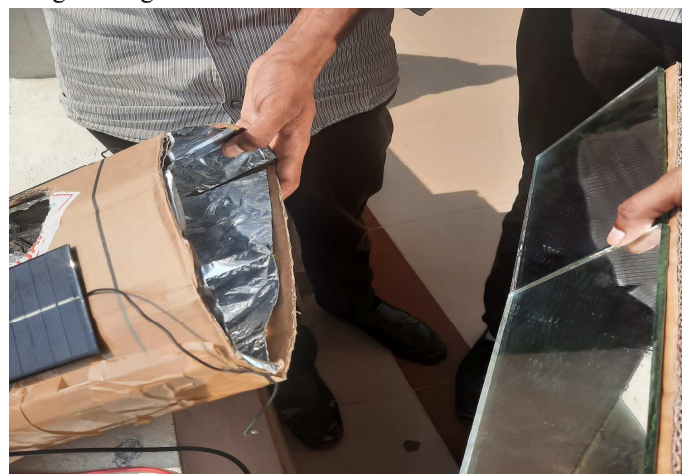
Figure 9. Top PV panel measurement under two mirror design arrangement
