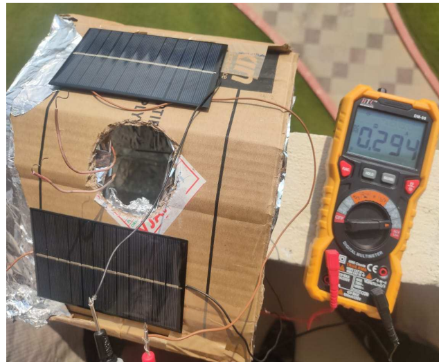
Figure 8. Top PV panel measurement under two mirror design arrangement
