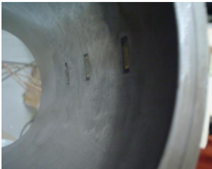
Figure 3: Liner Inner wall with installed Probes
