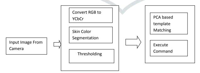
A) Input Camera Image: For the input the image is provided with help of camera. Cameras can webcam or mobile phone camera or depth camera depending on our requirement.
