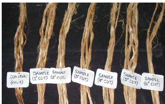
Fig. 1: Different samples (leaving 1"-6" of basal parts in the soil) of jute Fibre and their percent cutting
