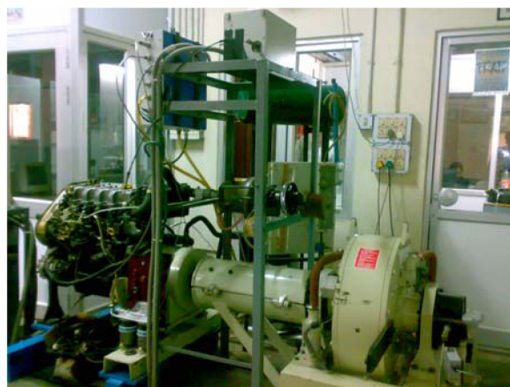
Figure 4. Experimental Setup of IDI Engine for Performance and Emissions
