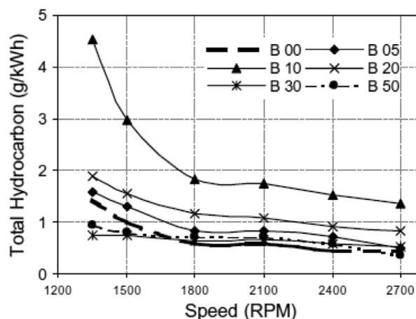
**Fig. 16.** THC emissions from biodiesel blends (Reprinted from [150], with permission of SAE).
