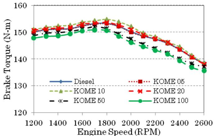
Fig. 8. Speed–torque characteristics for Karanja biodiesel blends (Reprinted from [152], with permission of Elsevier).
