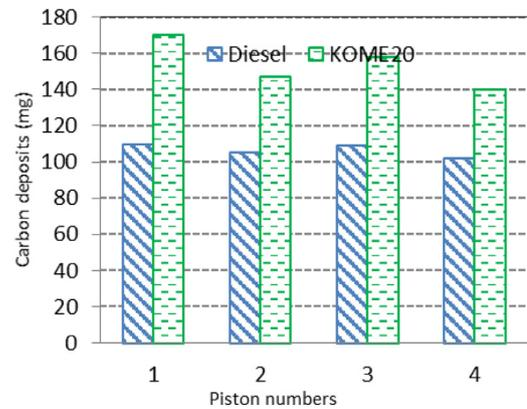
**Fig. 28.** Carbon deposits on the piston top of mineral diesel and B20 fueled engines (Reprinted from [292], with permission of Elsevier).
