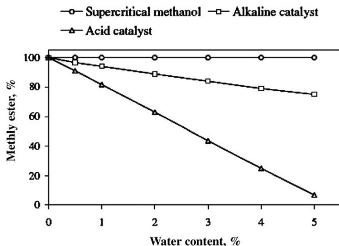
Fig. 4. Methyl esters yield vs. water content in various transesterification processes (Reprinted from [119], with permission of Sila Science Publications).
