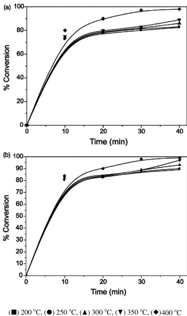
Fig. 5. Supercritical alcoholysis using (a) methanol (b) ethanol at different reaction temperatures (Reprinted from [124], with permission of Elsevier).
