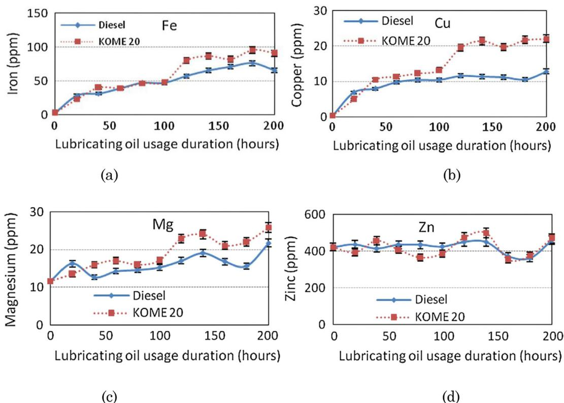
Fig. 30. Variation of trace metals in lubricating oil in a 200 h test (Reprinted from [313], with permission of Elsevier).
