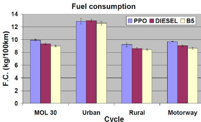
**Fig. 9.** Effect of 5% biodiesel blending on the brake specific fuel consumption (Reprinted from [168], with permission of SAE).
