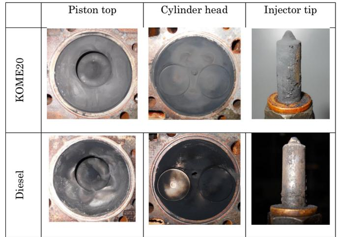
**Fig. 27.** Carbon deposits on the piston top, cylinder head and injector tip of mineral diesel and B20 fueled engines (Reprinted from [292], with permission of Elsevier).
