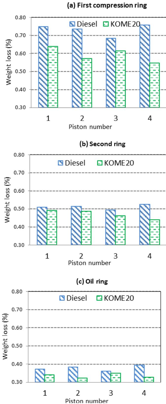
**Fig. 26.** Piston ring weight loss due to wear for (a) First compression ring (b) Second compression ring, and (c) Oil ring from mineral diesel and B20 fueled engines (Reprinted from [292], with permission of Elsevier).
