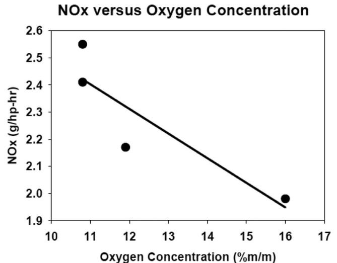
**Fig. 17.** NO<sub>x</sub> vs. oxygen concentration of the test fuel (Reprinted from [216], with permission of SAE).
