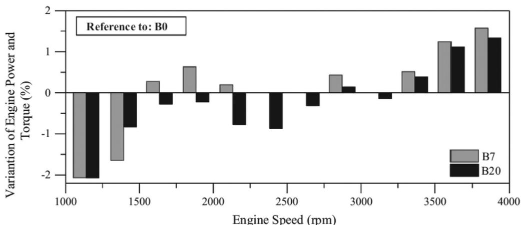
Fig. 7. Effect of biodiesel blending on the engine power and torque output (Reprinted from [151], with permission of Elsevier).
