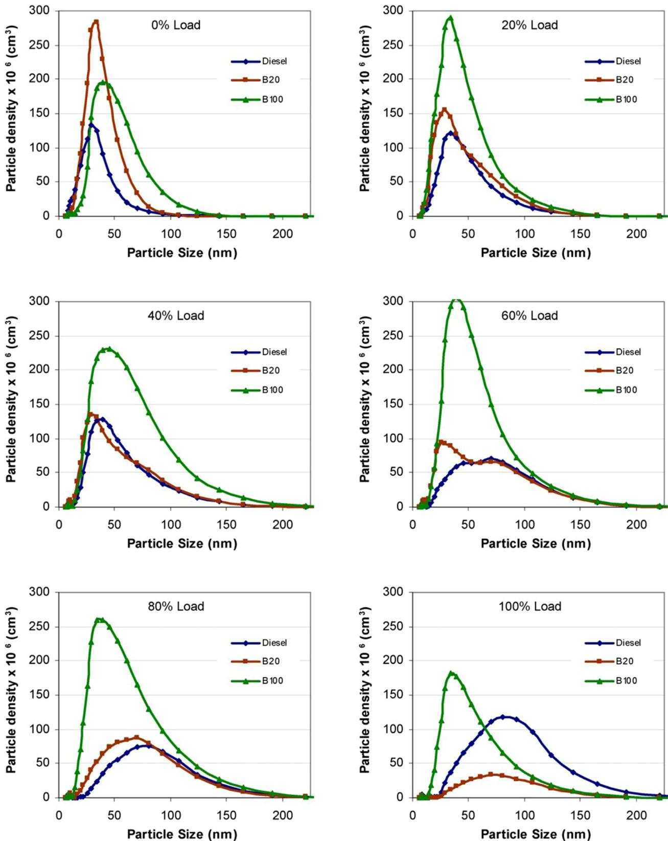
Fig. 21. Particle size-number distribution from biodiesel and blends at 1800 rpm for varying engine loads (Reprinted from [261], with permission of Elsevier).
