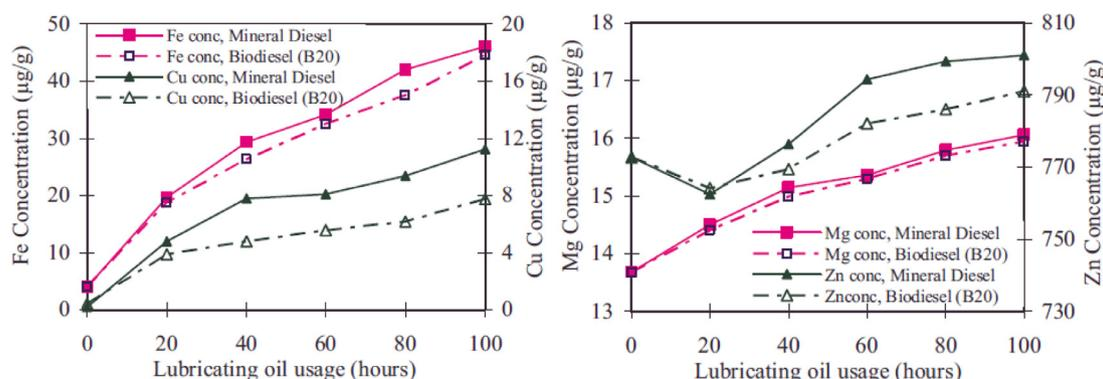
Fig. 29. Concentration of trace metals in lubricating oil in a 100 h test (Reprinted from [291], with permission of ASME).
