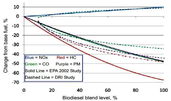
**Fig. 12.** Comparison of biodiesel engine emissions with EPA study (2002) (Reprinted from [187], with permission of SAE).
