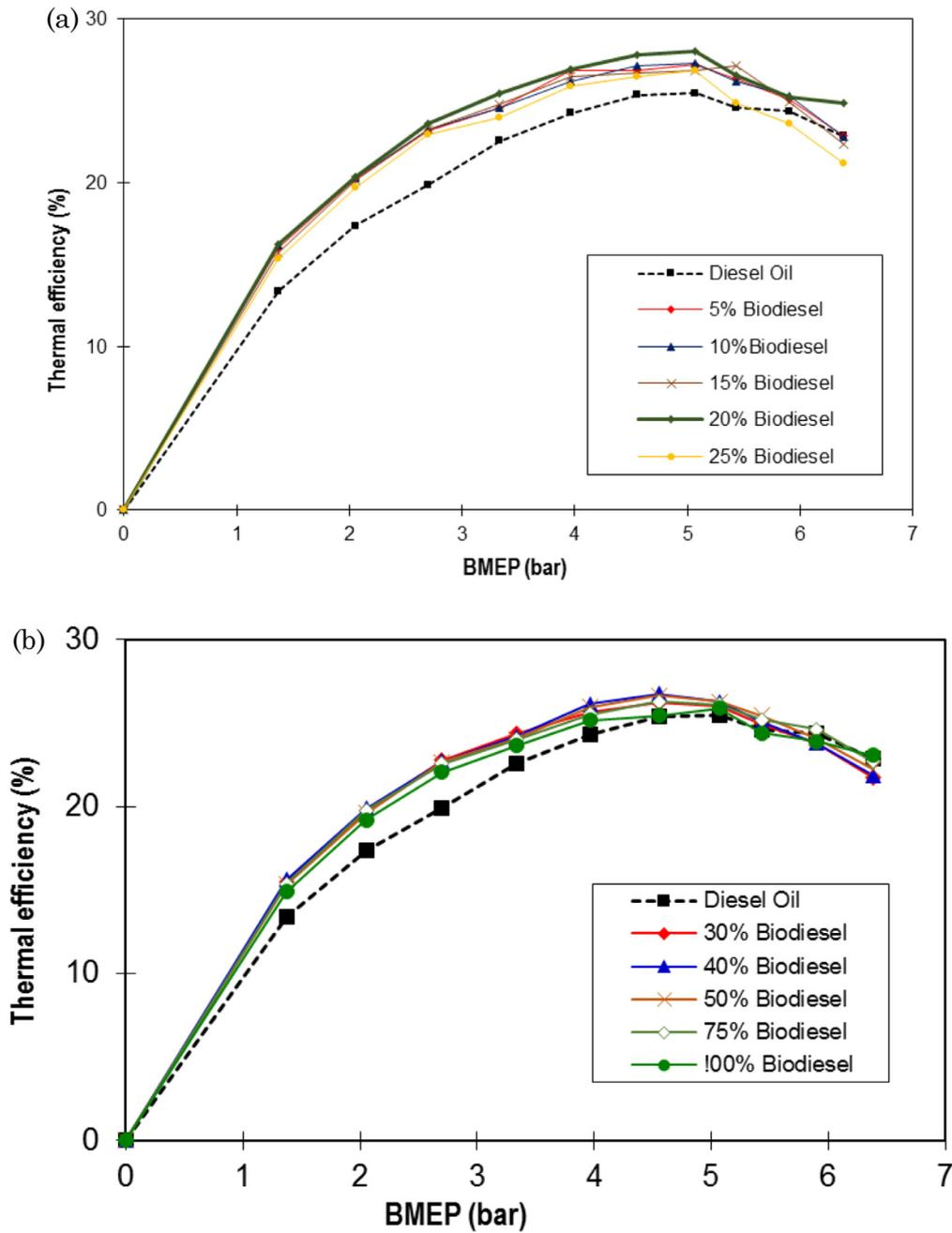
Fig. 10. Thermal efficiency vs. BMEP for (a) lower and (b) higher biodiesel blends (Reprinted from [178], with permission of ASME).
