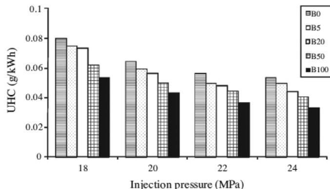
**Fig. 15.** Total hydrocarbon emissions vs. fuel injection pressure (Reprinted from [182], with permission of Elsevier).
