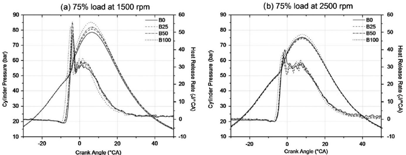
Fig. 23. Cylinder pressure and HRR of biodiesel/ blends compared to mineral diesel (Reprinted from [171], with permission of Elsevier).
