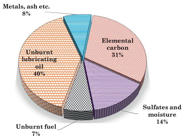
Fig. 20. Typical composition of diesel particulate matter (Reprinted from [7], with permission of Elsevier).
