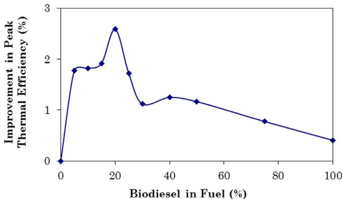
Fig. 11. Improvement in peak thermal efficiency vs. biodiesel blend concentration (Reprinted from [178], with permission of ASME).
