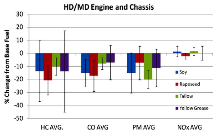
**Fig. 13.** Effects of biodiesel (B20) feedstocks on emissions (Reprinted from [187], with permission of SAE).
