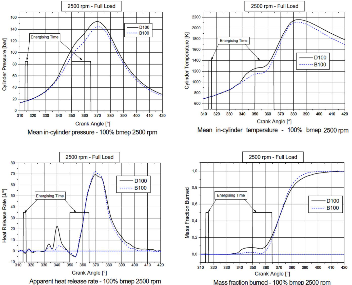
Fig. 24. (a) In-cylinder pressure, (b) In-cylinder temperature, (c) Heat release rate and (d) Mass fraction burned at 100% load, 2500 rpm in a CRDI HSDI engine using pilot injection (Reprinted from [155], with permission of SAE).
