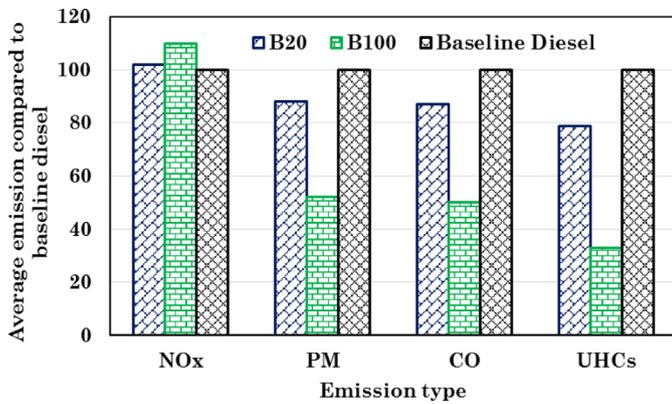
Fig. 14. Average emissions from biodiesel fuelled heavy-duty engines (Adapted from [186], with permission of EPA).
