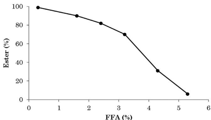
Fig. 3. Effect of FFA on biodiesel yield during alkali catalyzed transesterification (Reprinted from [64], with permission of Elsevier).
