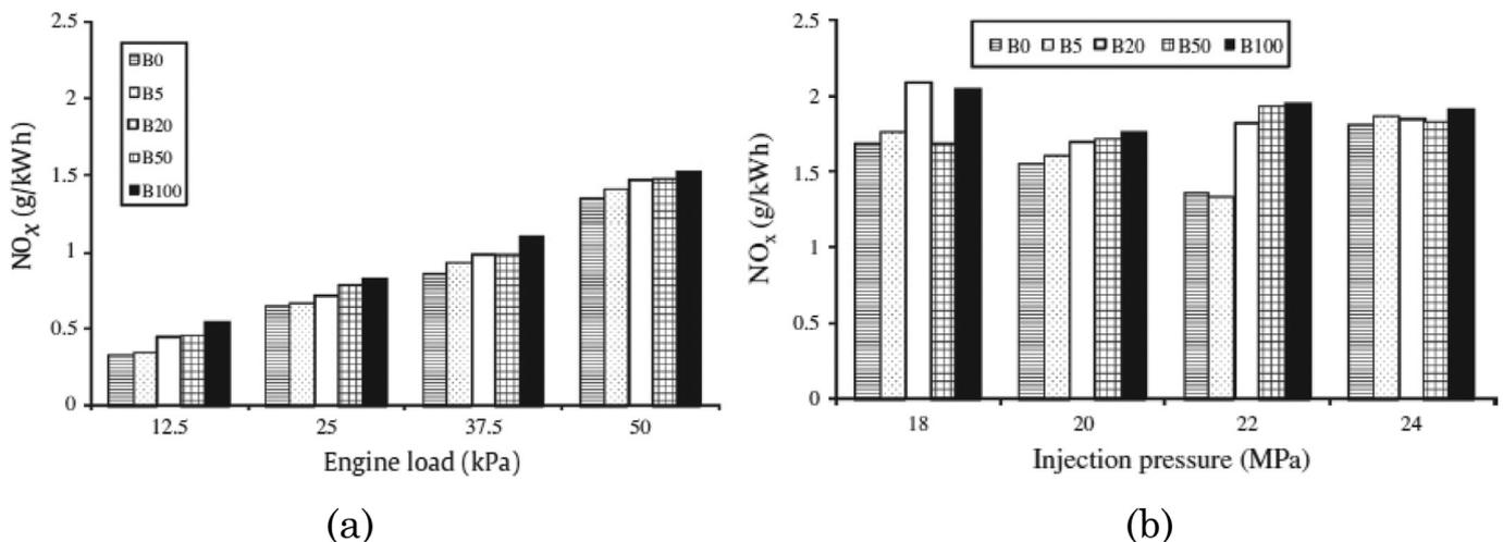
Fig. 19. (a) NOx emissions vs. engine load (b) NOx emissions vs. fuel injection pressure (Reprinted from [182], with permission of Elsevier).
