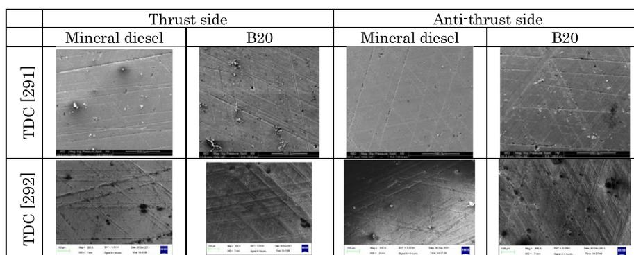
Fig. 25. SEM of liner surfaces for biodiesel and mineral diesel fueled engines (Reprinted from [291], with permission of ASME and from [292], with permission of Elsevier).
