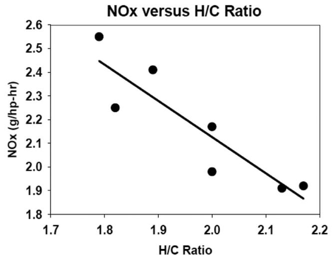
**Fig. 18.** NO<sub>x</sub> emissions vs. H/C ratio of the test fuel (Reprinted from [216], with permission of SAE).
