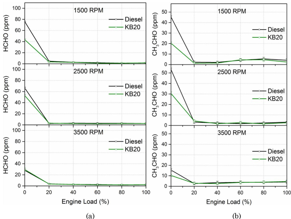
Fig. 22. Formaldehyde and Acetaldehyde emissions from biodiesel fueled engine (Reprinted from [267], with permission of SAE).
