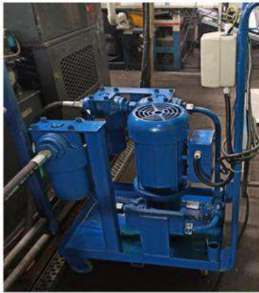
Used Filters of micron size up to 5 micron
