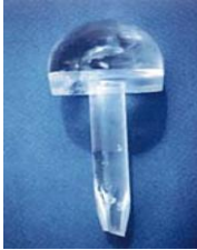
Figure 3: First Judet Stem Installed in 1946, Failed Due to Wear Debris of the Acrylic [5]
