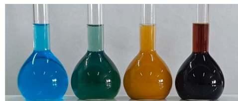
Fig. 1. Depiction of colour changes during nanofluid synthesis.
