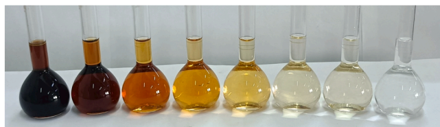
Fig. 7. Nanofluids with different particle weight fractions (0.215 %, 0.107 %, 0.054 %, 0.027 %, 0.013 %, 0.007 %, 0.003 % and 0.000 % from left to right, respectively).
