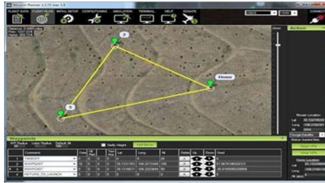
Fig.6. Mapping in ARDU Software for Autonomous Drone
