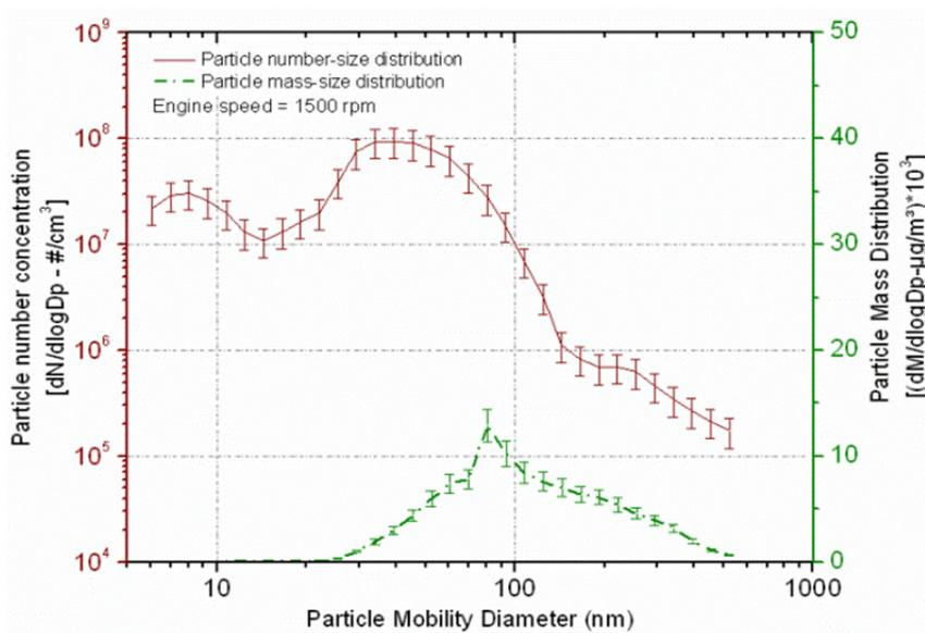
**Fig. 3.** Particle number-size distribution and particle mass-size distribution for heavy-duty CNG bus.
