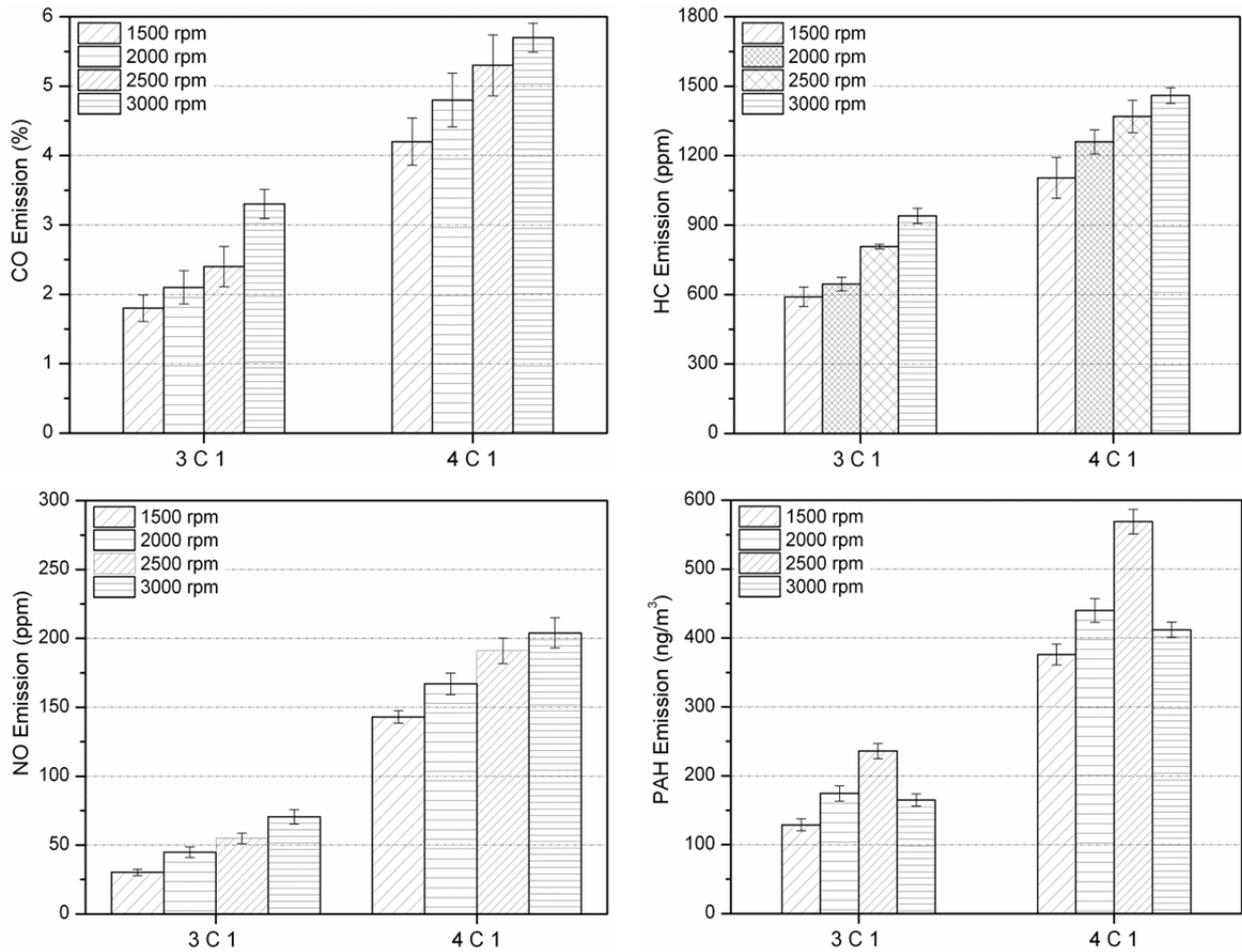
**Fig. 2.** Emissions of CO, HC, NO and particle bound PAHs from the CNG Tempo and CNG bus.
