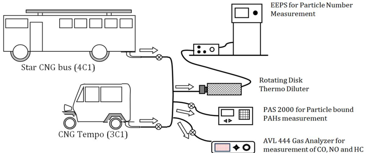
**Fig. 1.** Experimental setup for emission measurement from CNG fuelled vehicles.
