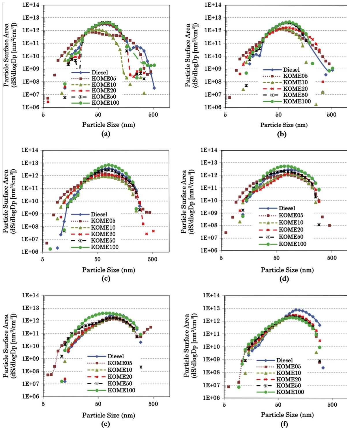
Fig. 4. Variation of particulate size-surface area distribution at 1800 rpm for BMEP of (a) 0.2 bar, (b) 1.4 bar, (c) 2.8 bar, (d) 4.2 bar, (e) 5.6 bar and (f) 6.8 bar.
