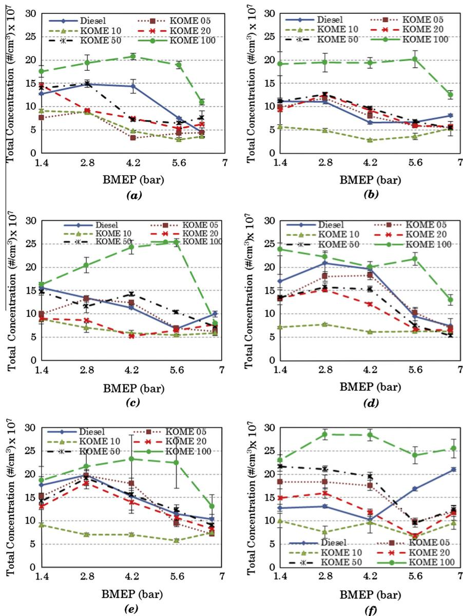
Fig. 7. Variation of particulate total number concentration of Karanja biodiesel and blends vis-à-vis mineral diesel at (a) 1200, (b) 1500, (c) 1800, (d) 2100, (e) 2400 and (f) 2600 rpm engine speed.
