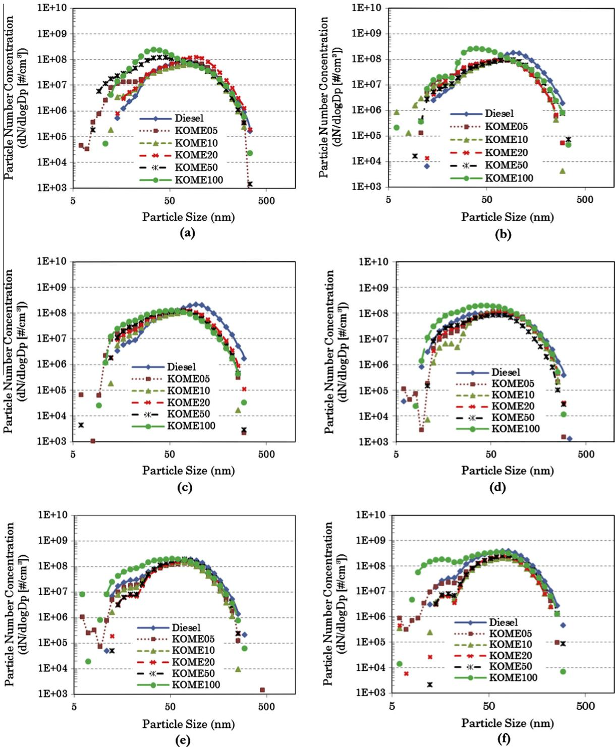
Fig. 3. Variation of particulate size-number distribution at 6.8 bar BMEP at (a) 1200 rpm, (b) 1500 rpm, (c) 1800 rpm, (d) 2100 rpm, (e) 2400 rpm and (f) 2600 rpm.
