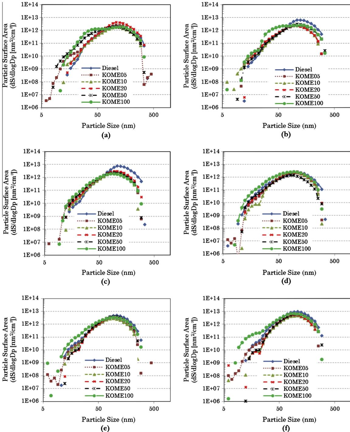
Fig. 5. Variation of particulate size-surface area distribution at 6.8 bar BMEP for engine speed of (a) 1200 rpm, (b) 1500 rpm, (c) 1800 rpm, (d) 2100 rpm, (e) 2400 rpm, and (f) 2600 rpm.
