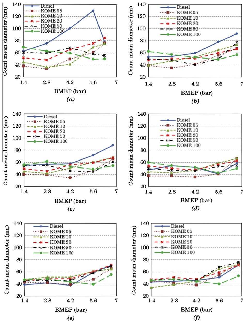
Fig. 6. Variation of particulate count mean diameter for Karanja biodiesel and blends vis-à-vis mineral diesel at (a) 1200, (b) 1500, (c) 1800, (d) 2100, (e) 2400 and (f) 2600 rpm engine speed.
