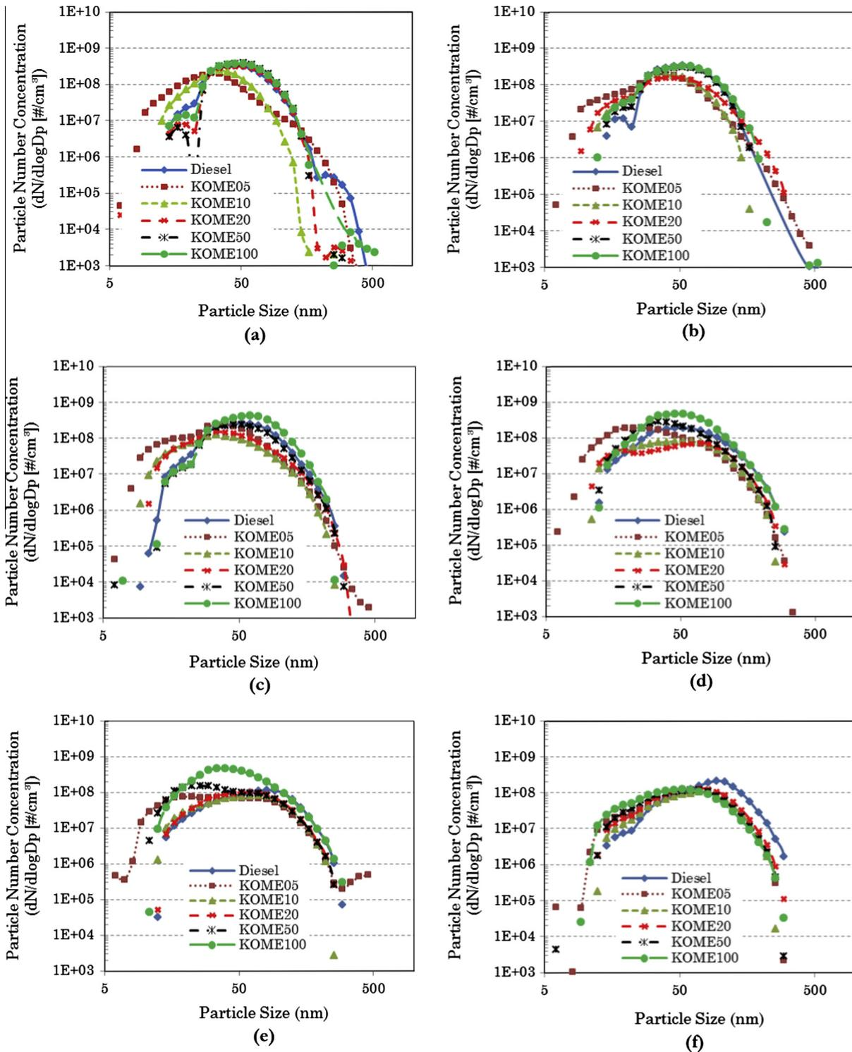
**Fig. 2.** Variation of particulate size-number distribution at BMEP of (a) 0.2 bar, (b) 1.4 bar, (c) 2.8 bar, (d) 4.2 bar, (e) 5.6 bar and (f) 6.8 bar at 1800 rpm.
