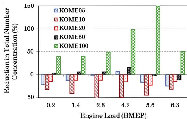
Fig. 8. Average reduction in total particle number concentration for Karanja biodiesel blends with respect to diesel at different engine loads.
