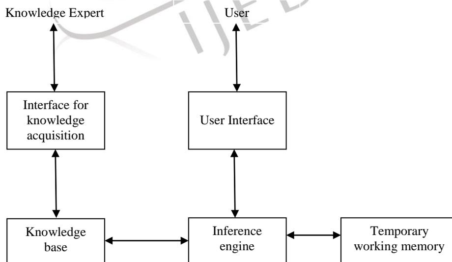
Figure 1: Components of Rule-Based Expert System
