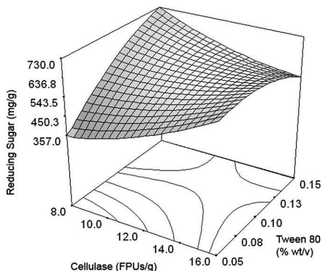
Fig. 1B. Response surface plot showing interaction effects of Cellulase & Tween 80.
