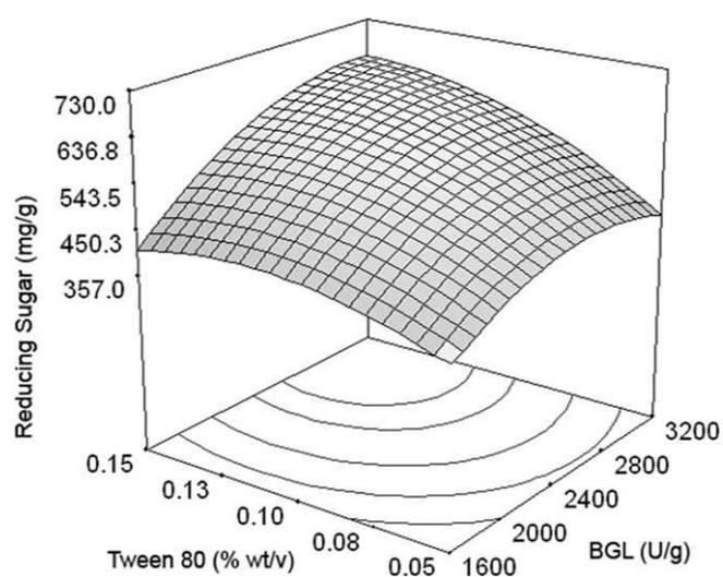
Fig. 1C. Response surface plot showing interaction effects of BGL and Tween 80.
